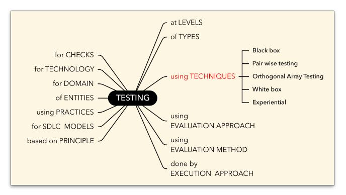
Test LEVELS, TYPES & TECHNIQUES are orthogonal i.e technique(s) is/are used to design test scenarios/cases for a type of test that is performed as part of a test level.
